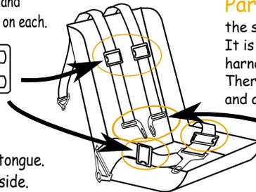
**Part 5** goes on the end of the shoulder harnesses. It is what connects the harnesses to the lap belt. There is a right-hand one and a left-hand one.
