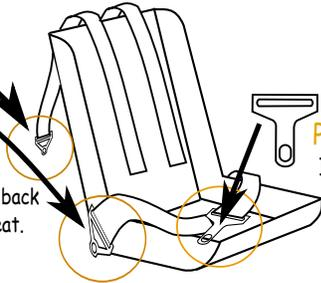
**Part 3** is the length adjustment component of the belts and harnesses. There is one on each.
